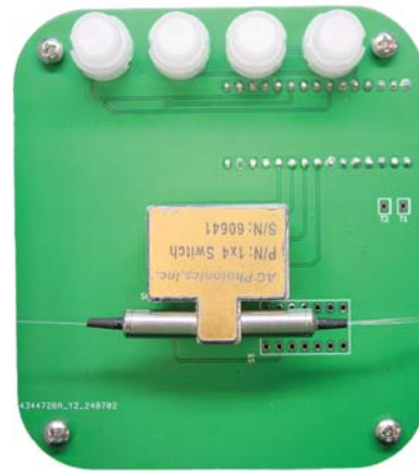
Figure 6: 1x4 mechanical switch mounted on the evaluation board.
