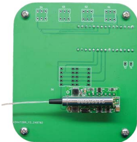
Figure 7: MEMS switch mounted on the evaluation board.
