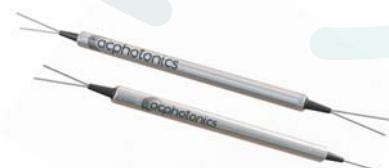
ACP's Polarization insensitive optical circulator utilizes proprietary designs and metal bonding micro optics packaging. It provides low insertion loss, broad band high isolation, low PDL, excellent temperature stability and optical path epoxy free. It can be used for wavelength add/drop, dispersion compensation and EDFA application.
